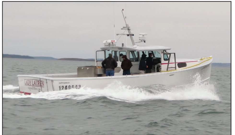
LADY LAUREN, a 38 Calvin Beal powered with a FPT C90 550 was launched at Bass Harbor. The boat was finished by Mike Light of Light Fiberglass in Corea. She has a Twin Disc 2.5:1 gear to a 32 x 34-inch propeller. She cruised at 21.5 knots and topped out at 23 knots. Her owner was extremely pleased with the boat and her speed. He was also pleased with the fuel consumption of just 17.5 gallons at cruising speed. It was also thought that if they add sprayrails she could gain about 5 mph to her cruising speed.
